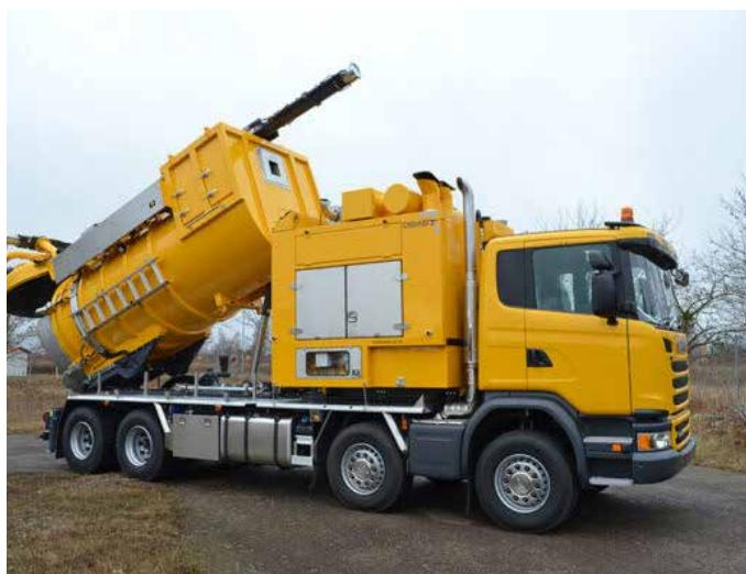
**DISAB Centurion™ LN20 is a truck mounted unit that can transport bulk materials and liquids by vacuum or overpressure through a hose system with a diameter up to 200 mm.**
