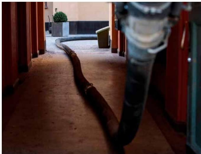
**DISAB Centurion™ LN14 is a truck mounted unit that can transport bulk materials by vacuum through a hose system with a diameter up to 200 mm.**
